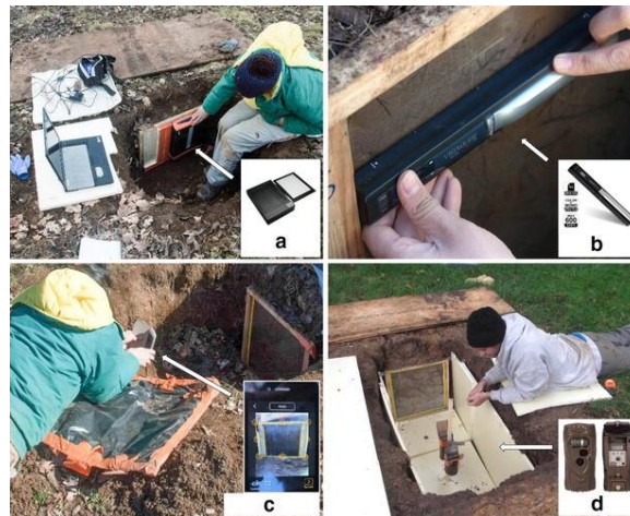
Fig: 2 a) flatbed scanner, b) handheld scanner, c) smartphone scanning application, d) time-lapse camera and rhizotron were placed into insulated boxes to prevent from external temperature variations.
